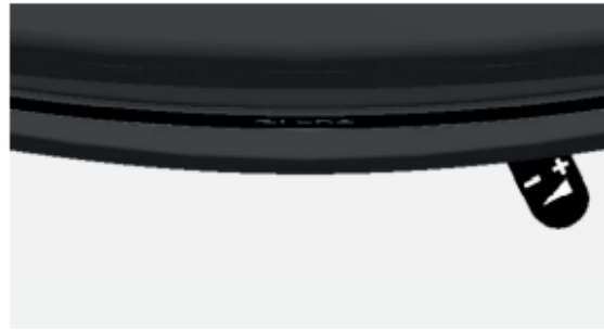
Combustion air completely open, handle on the far right
